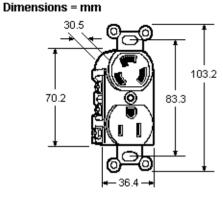
Combination Straight Blade and Locking Receptacles, 125 Volt 15 Amp, NEMA 5-15R and L5-15R, 2-Pole 3-Wire Grounded, UL Listed to meet/exceed UL 498 standards (UL File #E13399), CSA Certified (CSA File #LR406).
