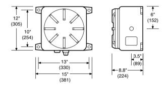
Includes clearance holes for mounting with 1/2" bolts.
