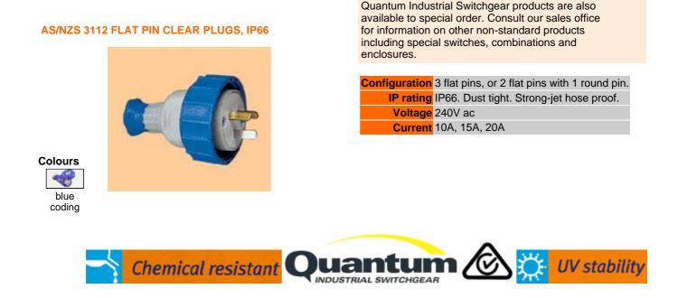
Clear plug body facilitates visual safety inspection of wiring. Specially designed terminal housing enhances speed and ease of wiring up. A clamp securely holds the cable preventing it twisting or damaging connections.
