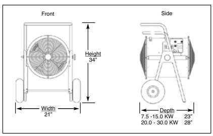
Note: All models are factory wired for 3 phase operation. Models designated 1 and 3 phase can be field wired for single phase operation.
