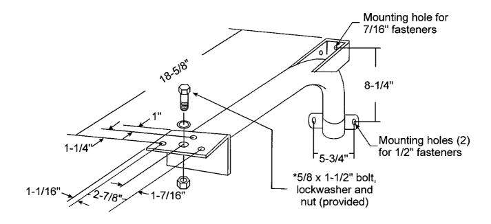
\*When using with TFM series yoke mounted luminaire, a 3/8" bolt, (2) lockwashers and nut must be used in placeof 5/8" bolt and lockwasher that is provided. Due to yoke design, the TFM will be off center when mounted.
