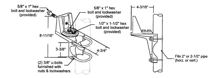
\*When using with TFM series yoke mounted luminaire, a 3/8" bolt, (2) lockwashers and nut must be used in placeof 5/8" bolt and lockwasher that is provided. Due to yoke design, the TFM will be off center when mounted.
