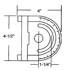
\*When using with TFM series yoke mounted luminaire, a 3/8" bolt, (2) lockwashers and nut must be used in placeof 5/8" bolt and lockwasher that is provided. Due to yoke design, the TFM will be off center when mounted.
