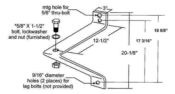
\*When using with TFM series yoke mounted luminaire, a 3/8" bolt, (2) lockwashers and nut must be used in placeof 5/8" bolt and lockwasher that is provided. Due to yoke design, the TFM will be off center when mounted.
