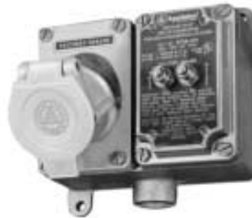
EFSR-GFI cover installed on two-gang EFD box together with U-Line 20A, 125VAC factory-sealed receptacle. Receptacle listed for Class I, Groups C and D, Class II, Groups F and G, and Class III.
